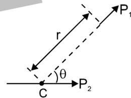
**G-7\*** An electric dipole is kept in the electric field produced by a point charge.
